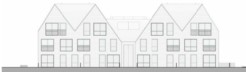
Fig 4. Proposed residential building – south elevation.
